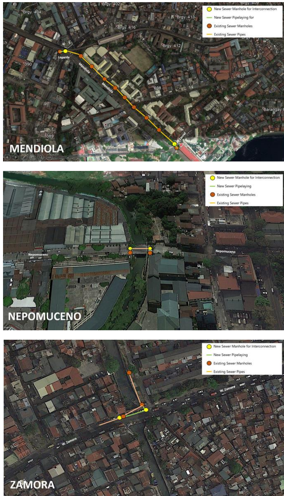
Figure 4.5: Sewer Line Replacement in Mendiola-Nepomuceno-Zamora
